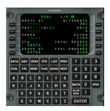
"Proceed" to use the FCDU to load the aircraft. Makes no difference if you select manual load or normal load. I prefer normal load. If you do reach the reconciliation screen after loading and it asks you to reconcile the load, select aircraft.
